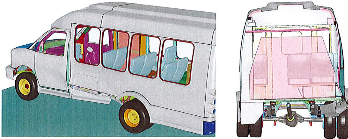
Figure 28: Final deformation of the bus body for the FE model with improved connections.
