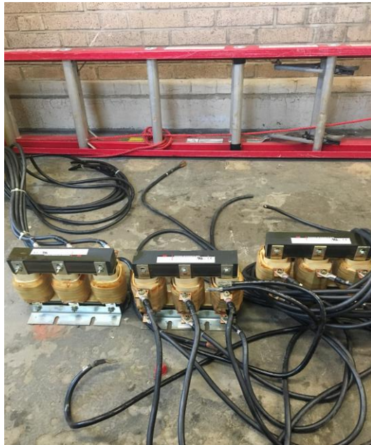
KLR Series Line Reactors Trans Coil Inc. (TCI) Model No. KLR 110ACB 3 Phase; 60 Hz; 600V Max.; 110 A Quantity: 3
