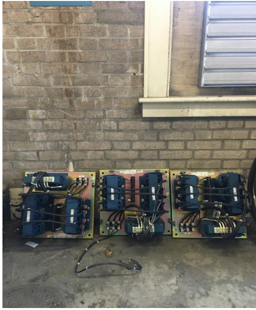
Harmonic Filters MTE Corporation CAT. No. M3-0050PD-12 50 HP; 3 Phase; 60 Hz; 480V Quantity: 3
