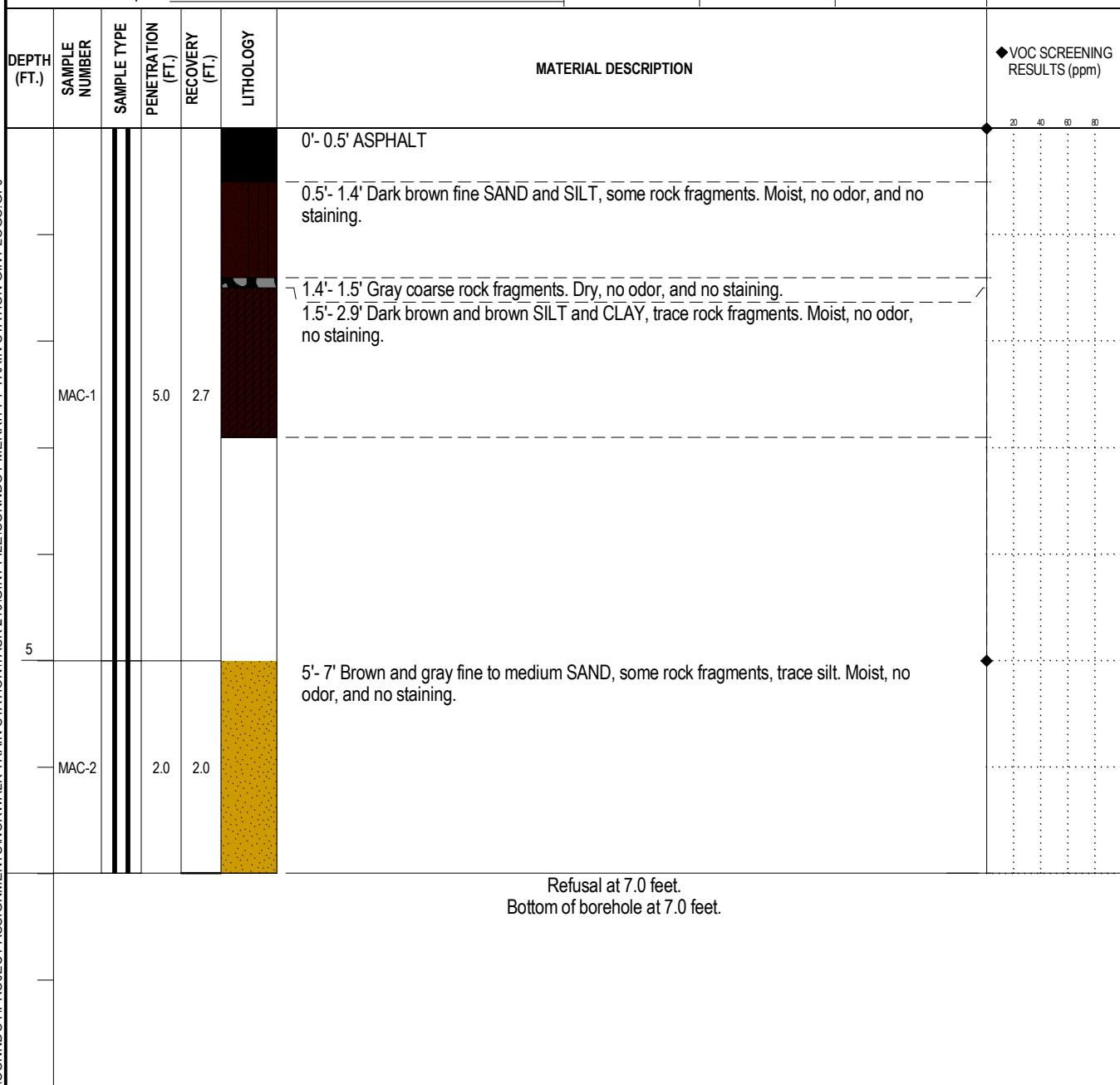
Notes: Collected sample SB-12 from 1' to 3' ftbg for VOCs, SVOCs, ETPH, PCB's, total and RCRA 8 metals.
