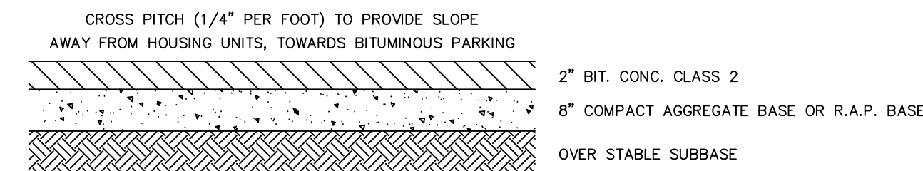
SIDEWALKS BITUMINOUS PAVEMENT DETAIL
