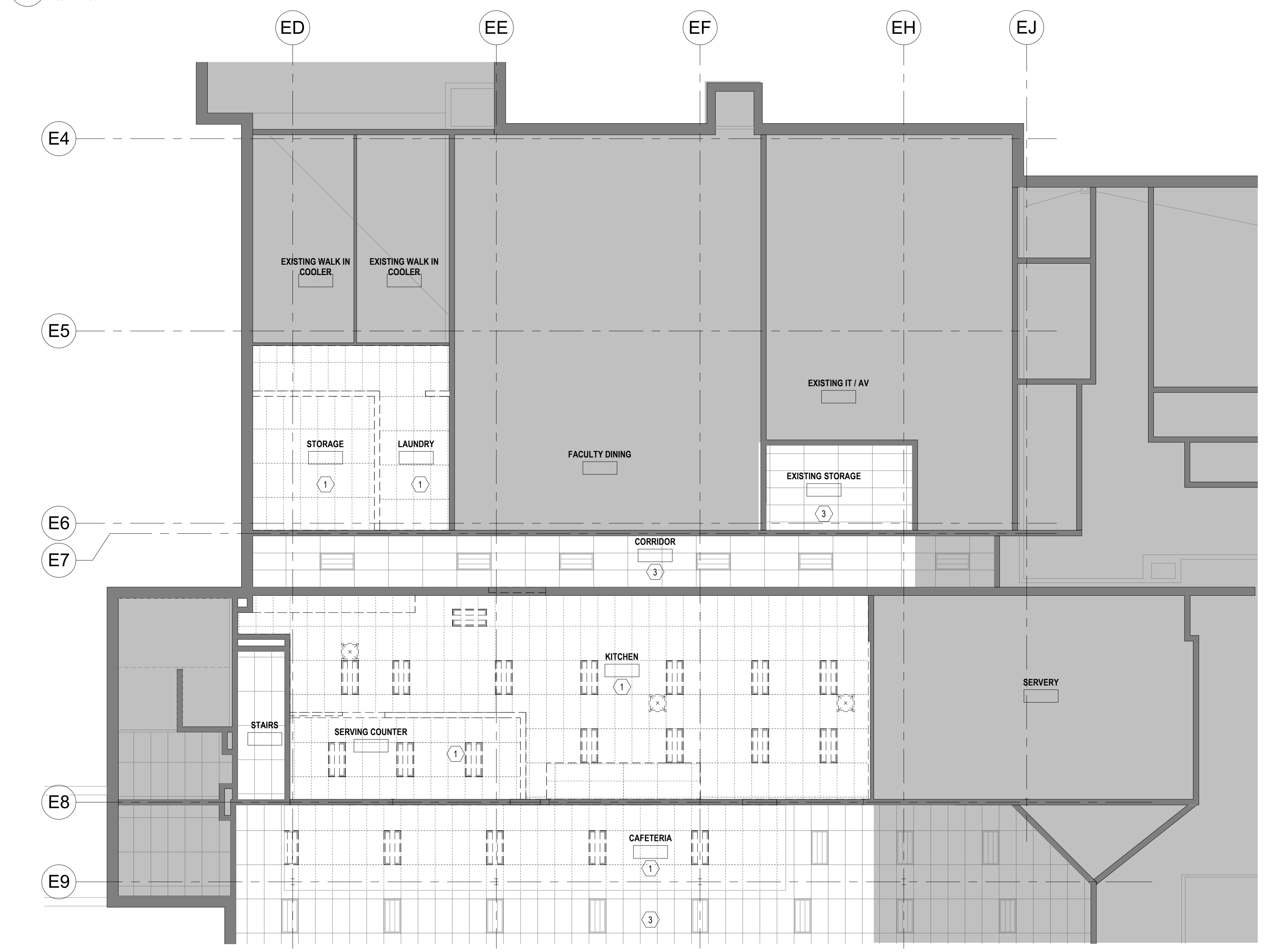
1 FIRST FLOOR DEMOLITION REFLECTED CEILING PLAN 1/8" = 1'-0"
