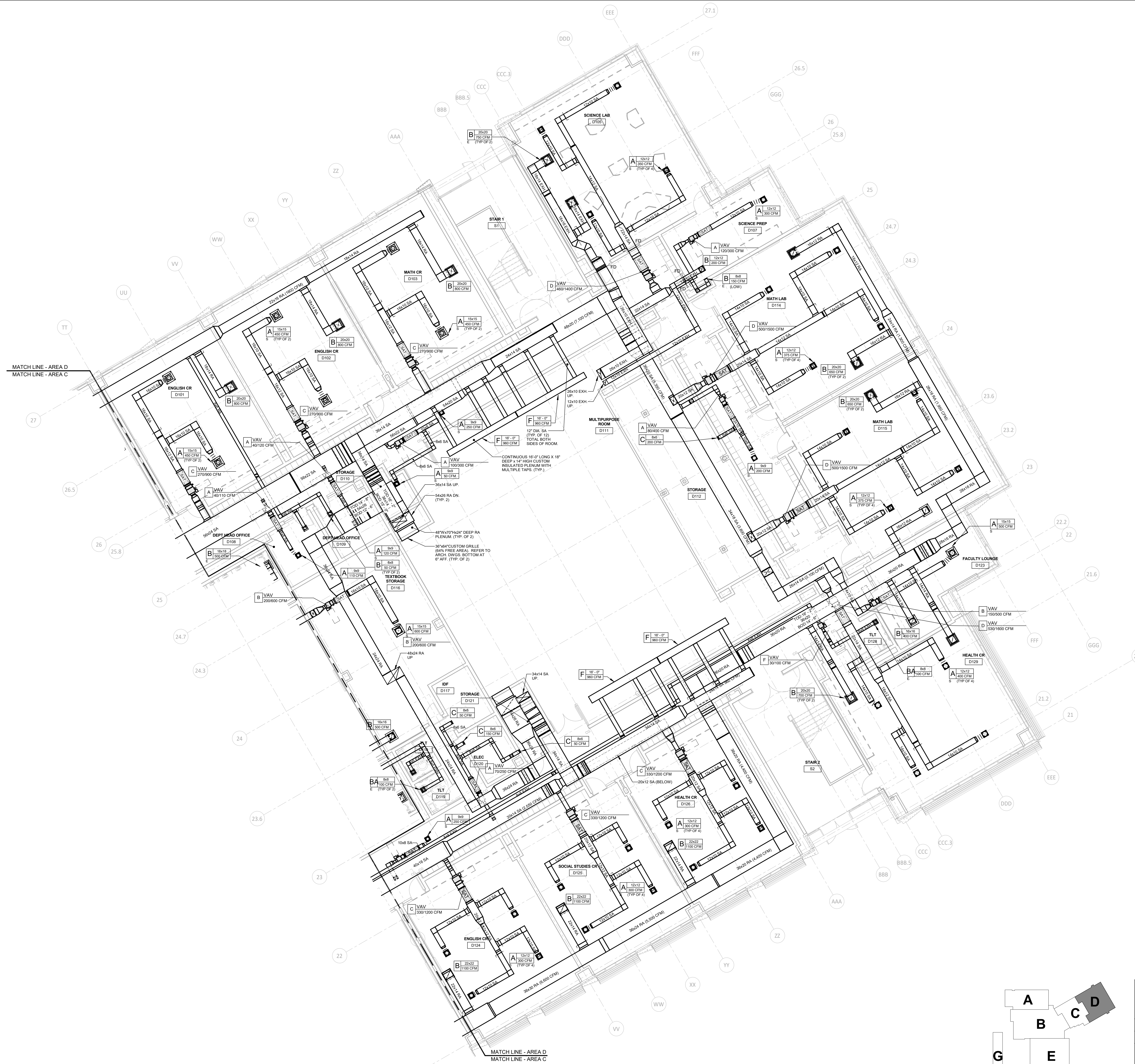
1 FIRST FLOOR MECHANICAL PLAN - AREA D 1/8" = 1'-0"
