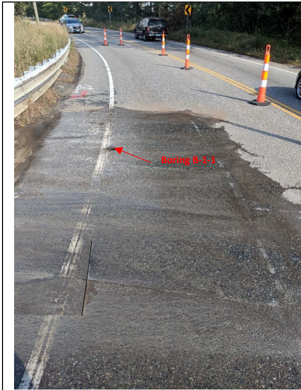
Bridge 02932, Test Pit T-1-1 (foreground) and T-1-2 (background). General view of asphalt cuts.
