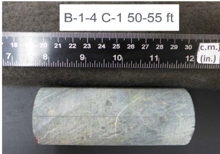
After cutting and grinding
