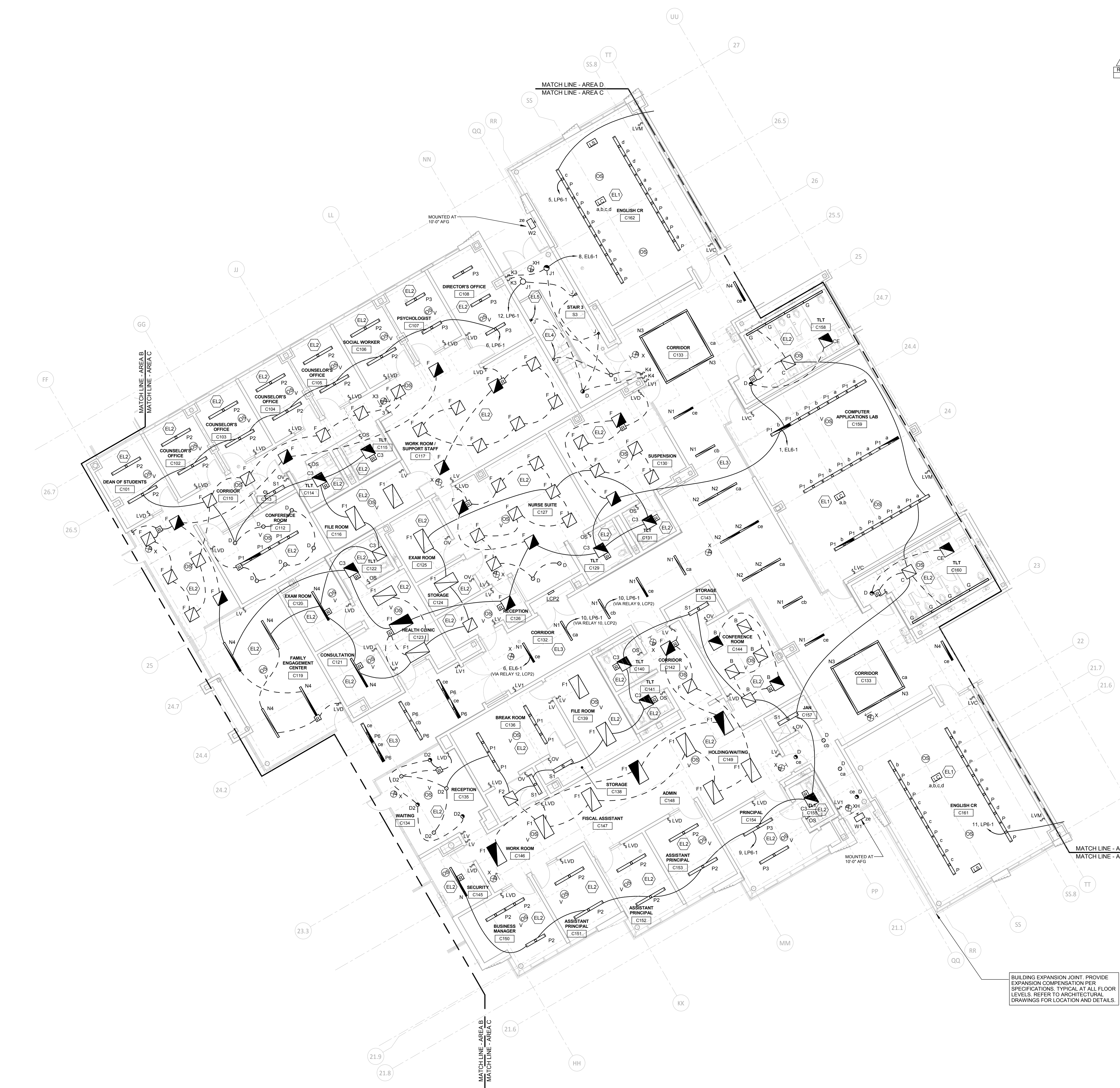
1 FIRST FLOOR LIGHTING PLAN - AREA C 1/8" = 1'-0"
