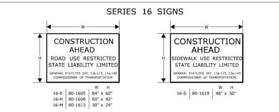
THE 16-S SIGN SHALL BE USED ON ALL PROJECTS THAT REQUIRE SIDEWALK RECONSTRUCTION OR RESTRICT PEDESTRIAN TRAVEL ON AN EXISTING SIDEWALK.
