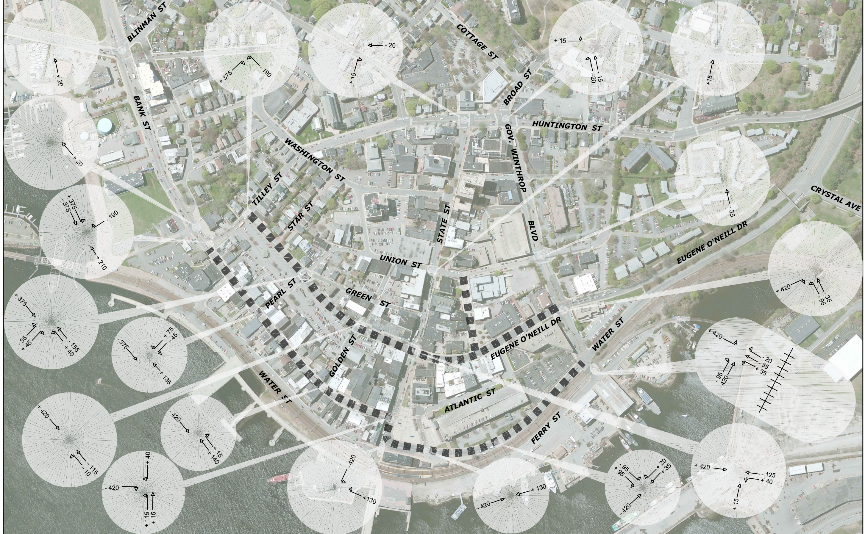
ONE-WAY TO TWO-WAY TRAFFIC VOLUMES RE-ROUTED FULL TWO-WAY SCENARIO - WEEKDAY PM PEAK HOUR DOWNTOWN TRANSPORTATION STUDY New London, Connecticut
