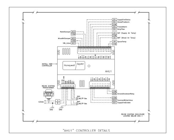
Install new Honeywell differential enthalpy sensor to terminal - COM – UI4 and UI5 Provide dual enthalpy control OA. Return air and CO2 control
