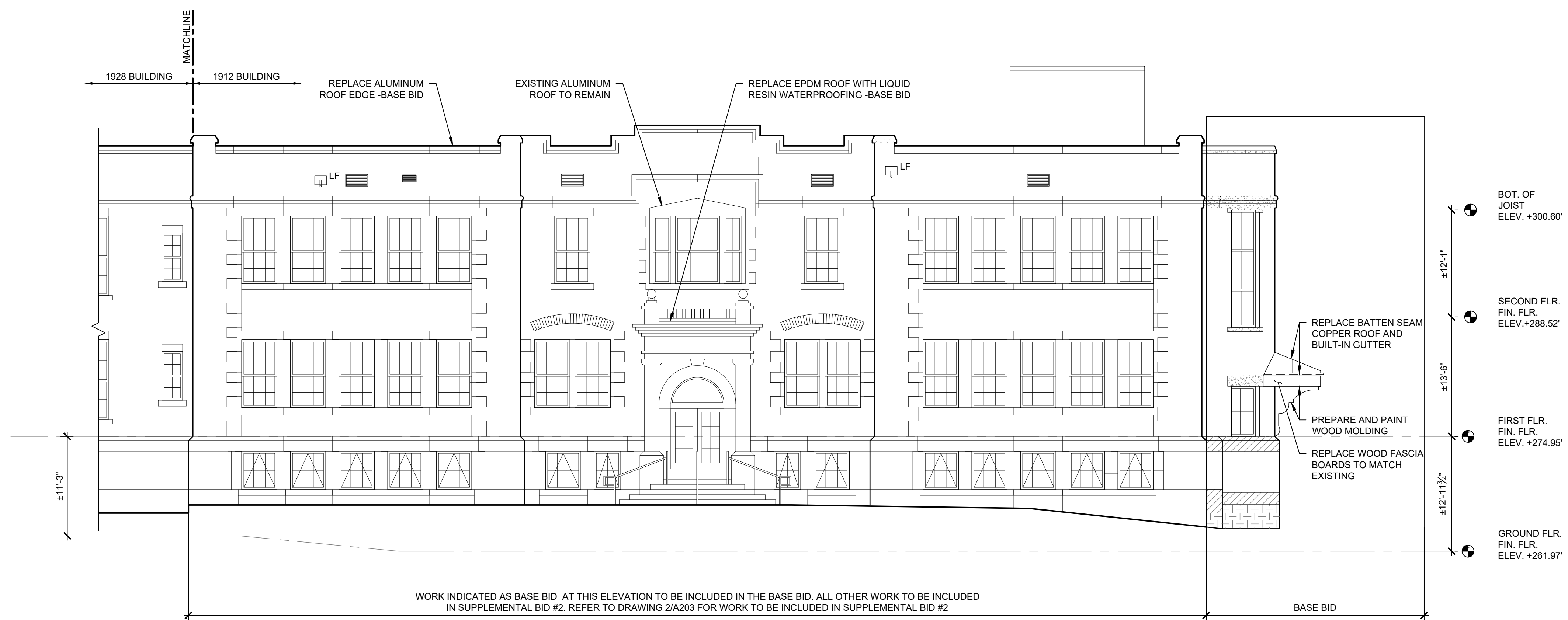
2 WEST ELEVATION - 1912 BUILDING BASE BID WORK SCALE: 1/8" = 1'-0"
