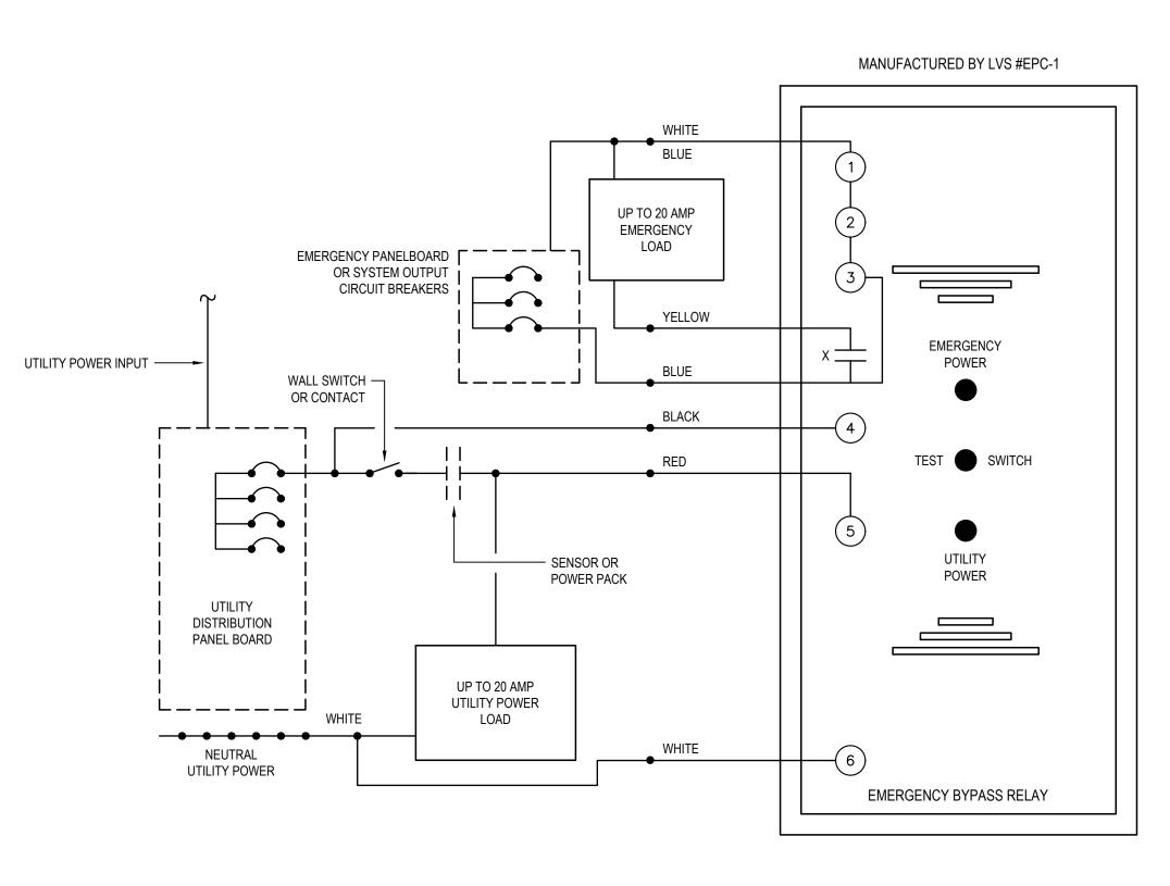
EMERGENCY LIGHTING BYPASS RELAY WIRING DIAGRAM E-6.1 SCALE: NONE
