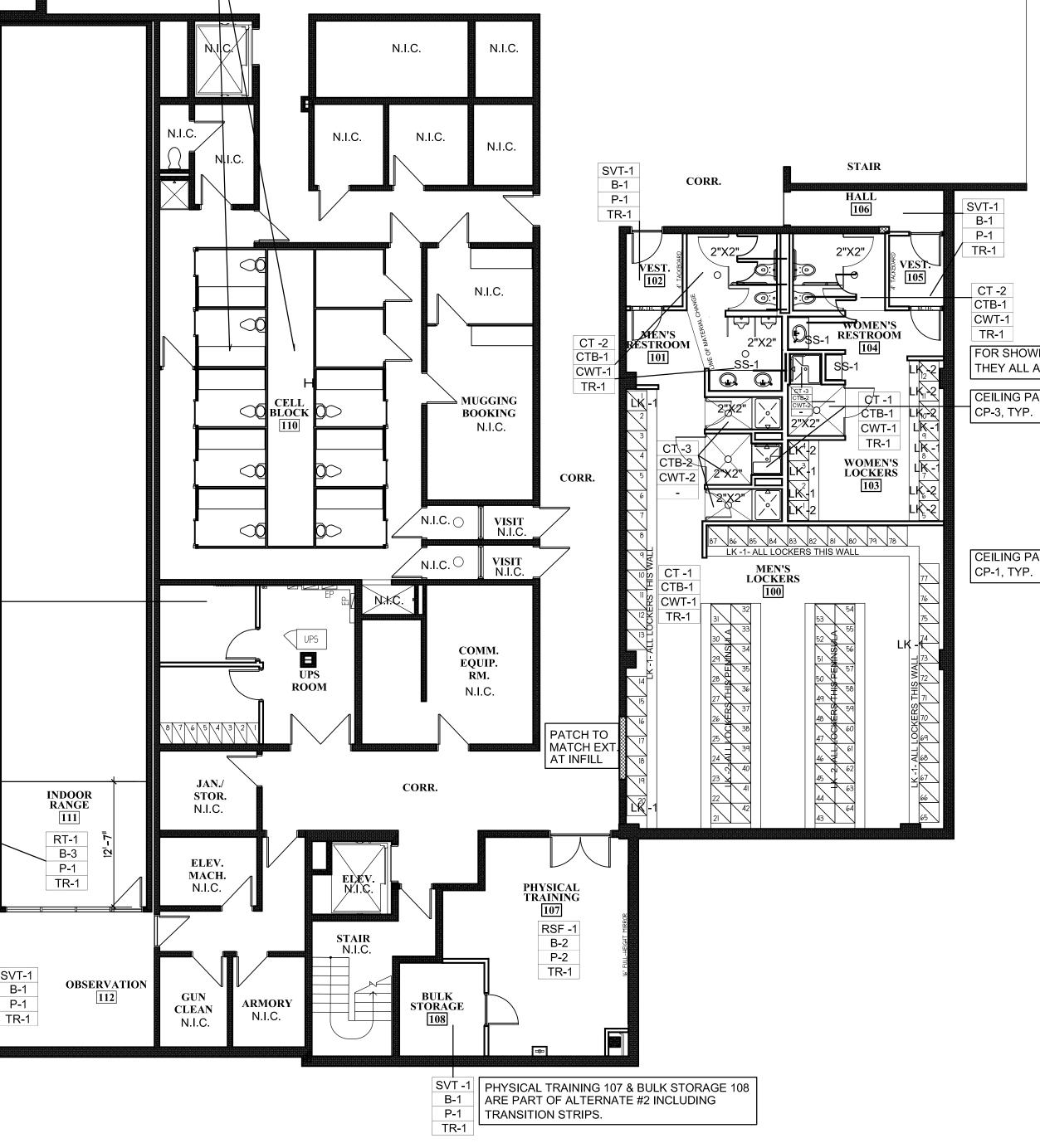
EACH CELL TO RECEIVE AN EPOXY PAINTED 30" HEIGHT CELL NUMBER, CENTERED ON WALL OPPOSITE SECURITY CAMERA, IN CONTRASTING COLOR.
