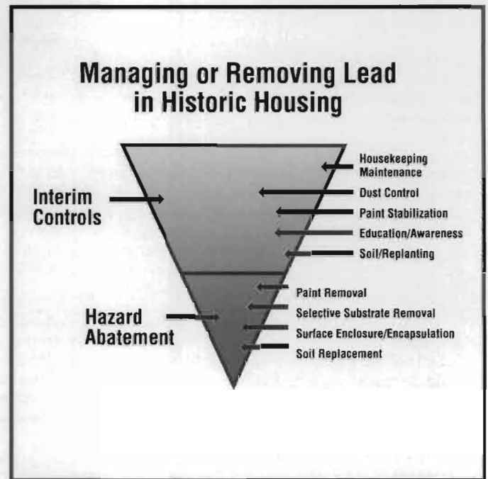
Figure 12. An inverted triangle makes the point that most of the nation's housing can be made lead-safe using interim control methods, such as dust control, paint stabilization, and good housekeeping. Shaded from light to dark, the lighter interim controls will generally not harm the historic materials. The darker, more aggressive controls, can be implemented with rehabilitation projects where paint removal, selective replacement of deteriorated elements, and encapsulation or enclosure are incorporated into other work.
