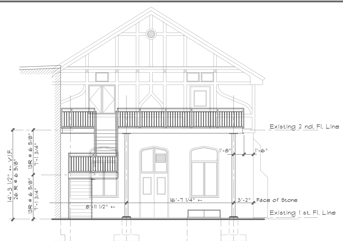
Elevation of New Exit Stair
