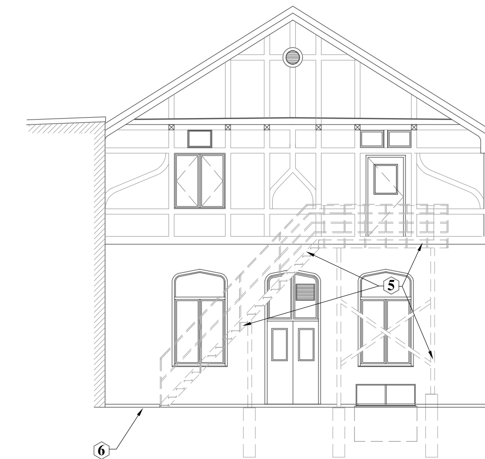
Rear Elevation at Fire Escape Showing Demo of Fire Escape
