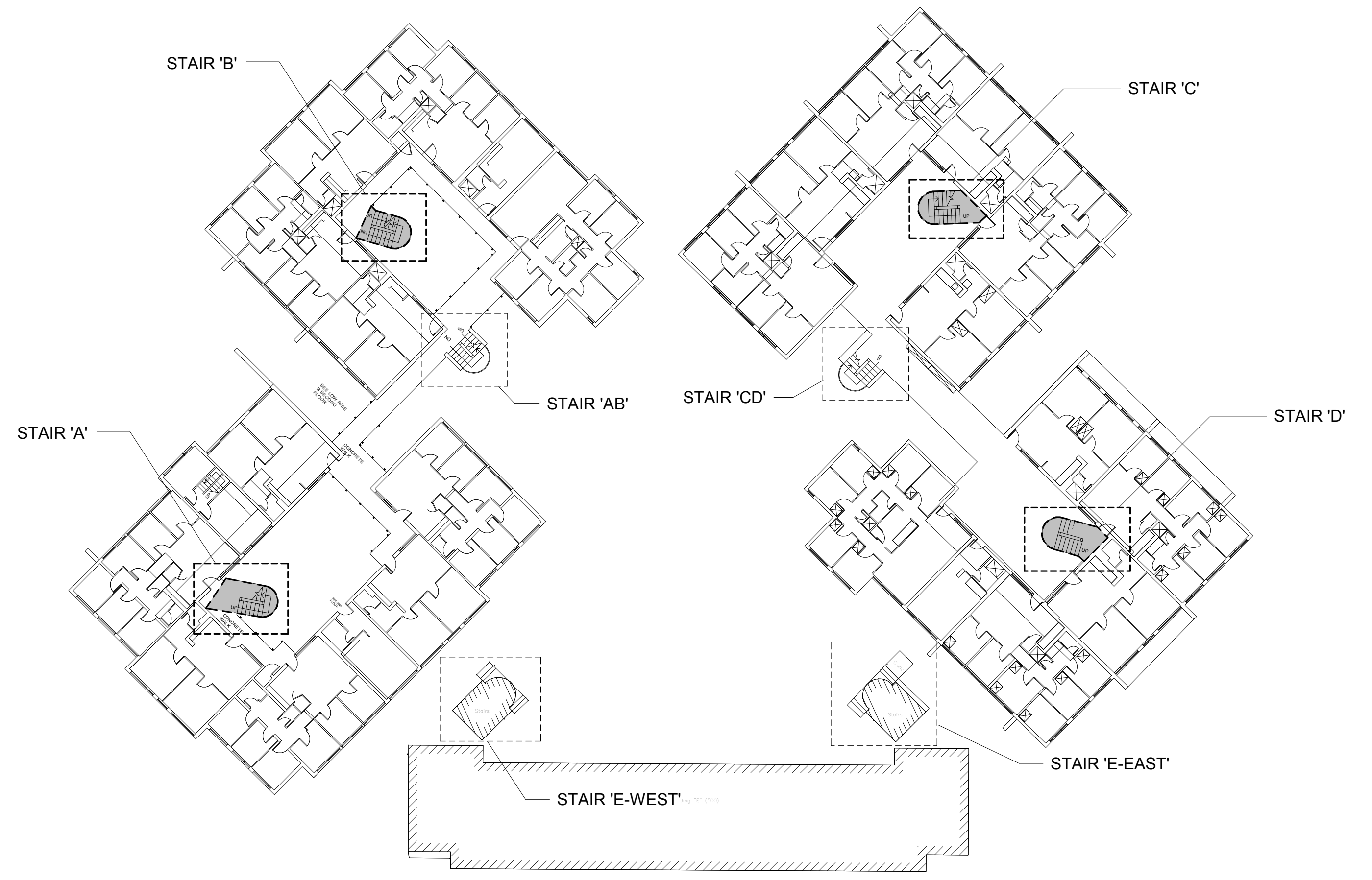
STAIR DEMOLITION PLAN
