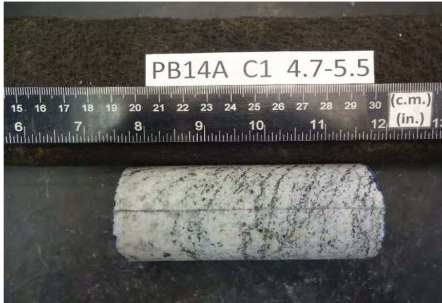
After cutting and grinding
