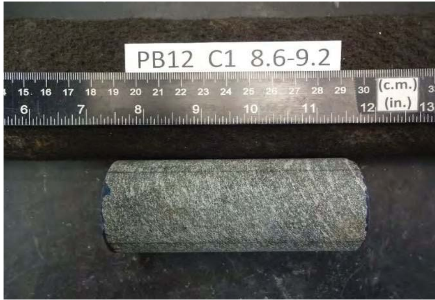
After cutting and grinding
